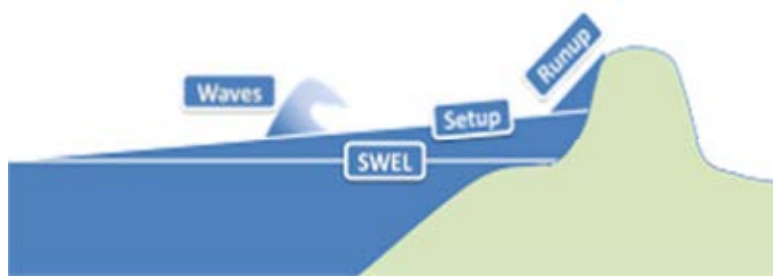
Figure 1: Coastal BFE includes storm surge, wave setup, overland wave heights or runup elevations.
